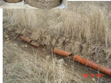
Tile failure: above-clay tile exposed, right-blow holes flagged in field, below: clay tile exposed in blow hole.
